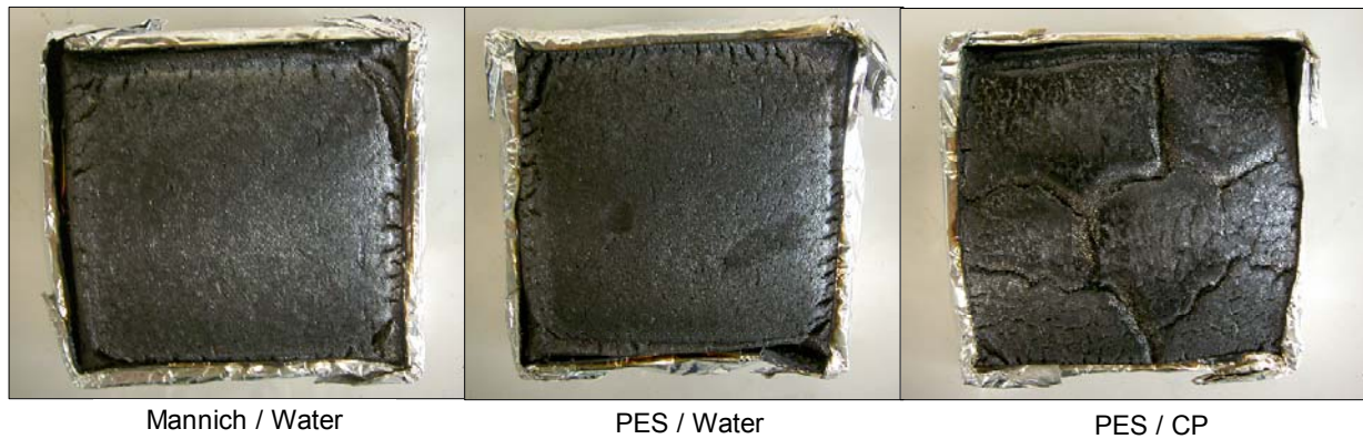
Figure 8. Appearance of test sample after cone calorimeter test
